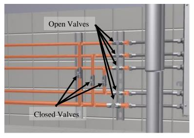
Figure 9 - Manifold Valve Settings - Normal
