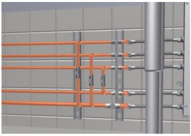
Figure 8 - Manifold Valve Settings - Flush
