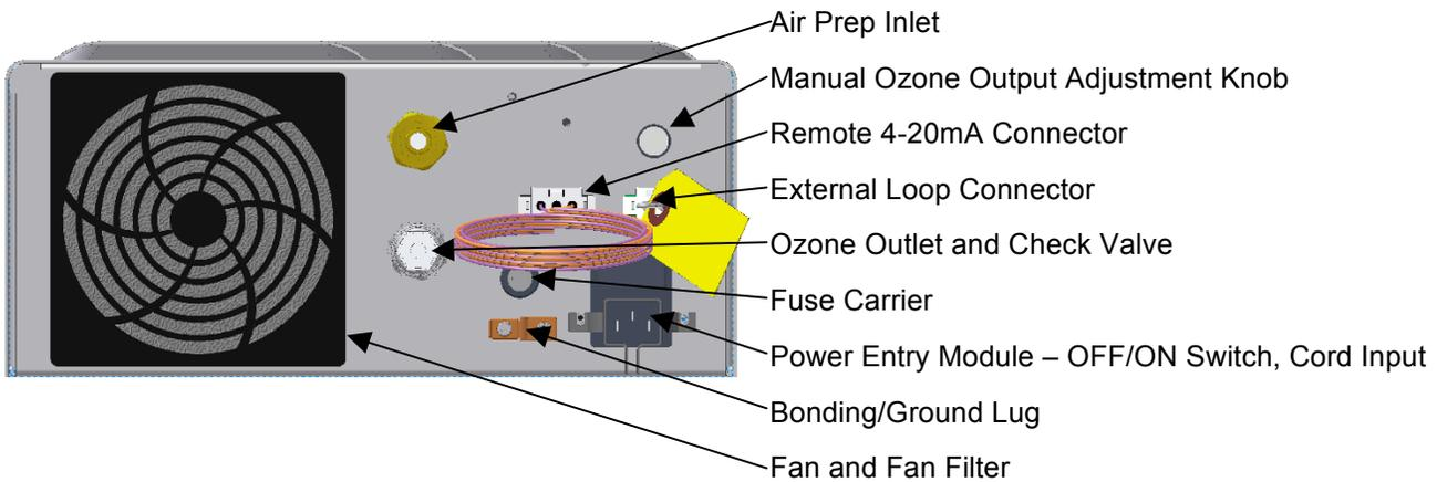
Shown: ClearWater Tech CD12 Ozone Generator (Wire harness omitted for clarity)
