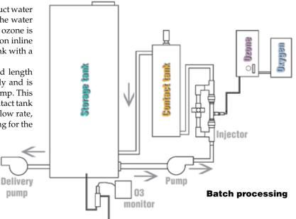
into the water stream circulating into the tank. In circulating the water, the whole tank is presumed to be exposed by the volume of water through the pump and Venturi system. Bubbling uses a small ozone generator and air pump to create ozone gas and push it through a diffusion stone into the storage tank.
