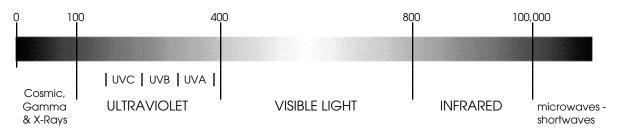
Figure 1 • Wavelengths in nm
