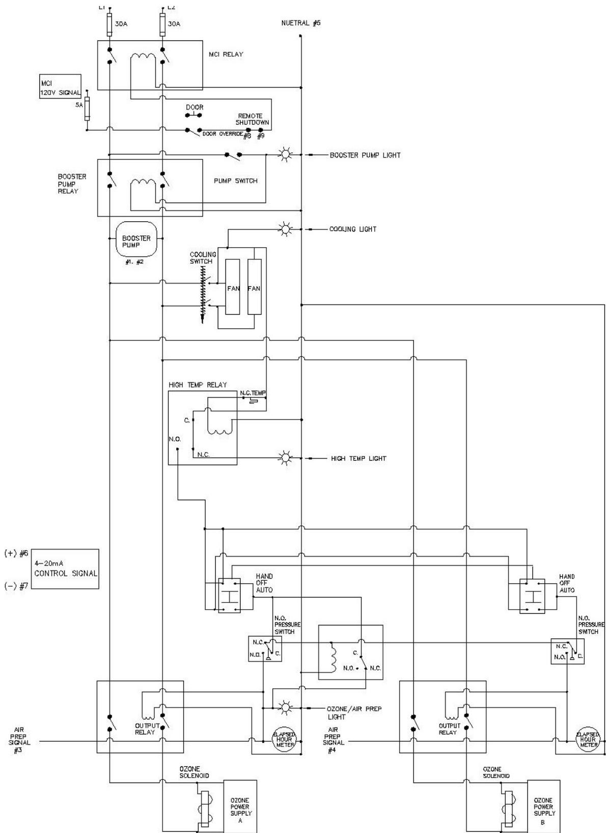
Shown: Electrical Schematic – CD8000P and CD12000P Line Side
